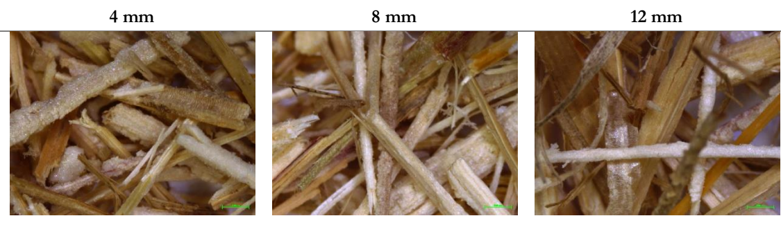
Figure 44. Miscanthus particles before densification (magnification 6.5×)
