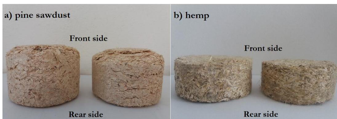
Figure 58. Briquettes of pine sawdust and hemp (8 mm) after the abrasion test
