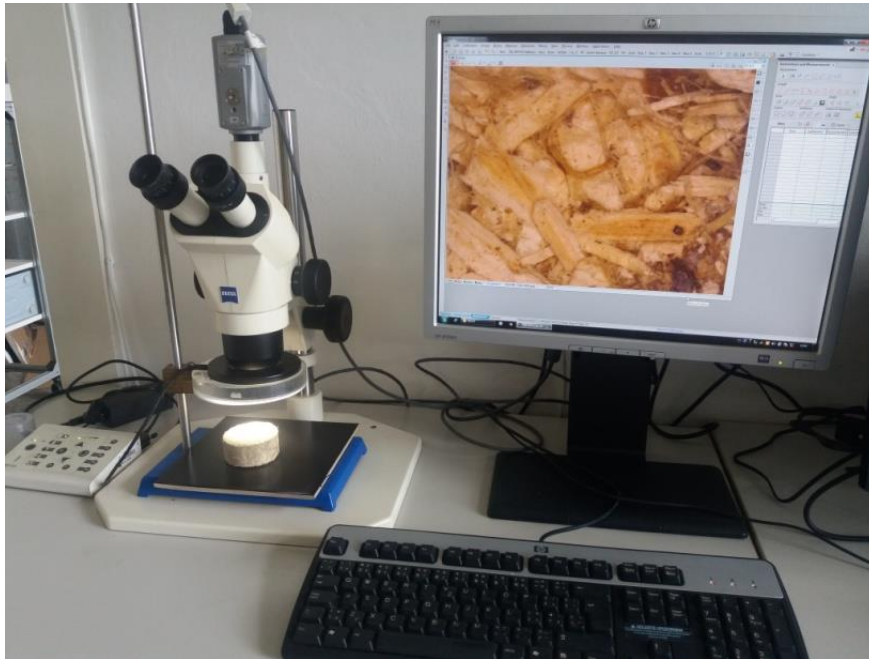
Figure 20. Equipment employed for macroscopic analysis of briquettes
