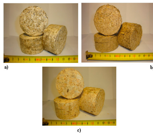
Figure 1. Produced briquettes made of different biomass sources: (a) hemp; (b) miscanthus; (c) pine sawdust.
