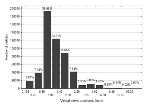
**Figure 2.** PSD of measured pine sawdust with max feret diameter ( $X_{max}$ ) as measuring algorithm (in mm).
