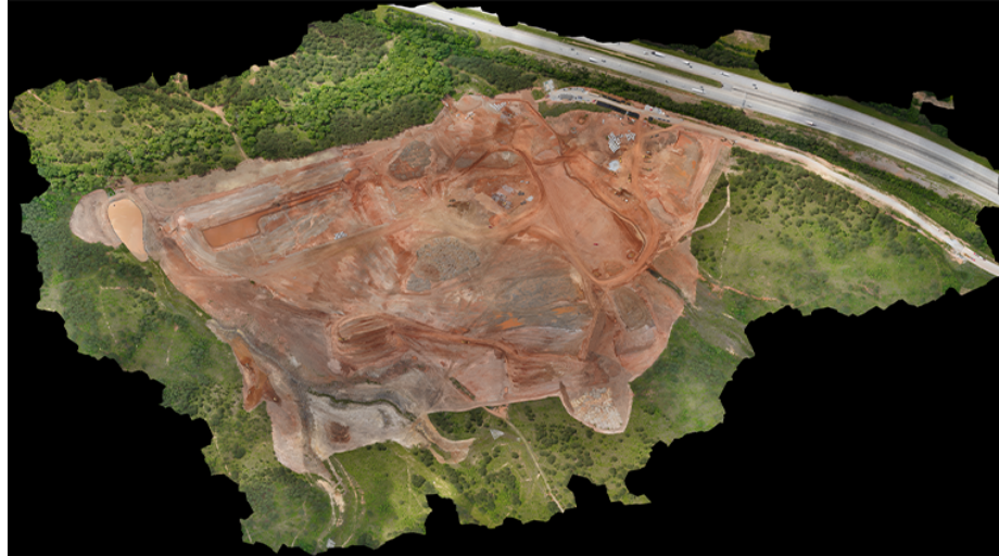
Figure 2.1: Bridgeport Moreland Construction Orthomosaic [19]
