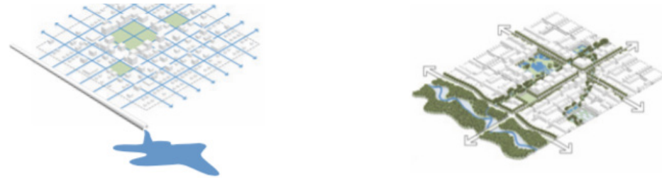
Figure 15: The above diagrams represent a North American approach to LID urbanism which replaces conventional urbanism (left) consisting of a “drain, direct, dispatch, approach by treating water on site and at the surface with an integrated LID (right) “slow, spread, soak” approach, as applied in the Vauban District (University of Arkansas Community Design Center, 2010).
