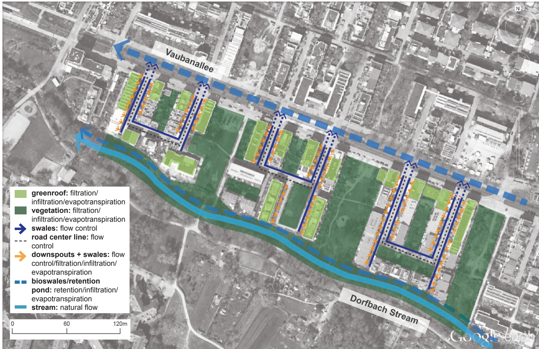
Figure 17: This diagram summarizes the general water management schemes on Site B as also represented with photographs and descriptions (Created by author, Original map data: Google Earth, 2016c).
