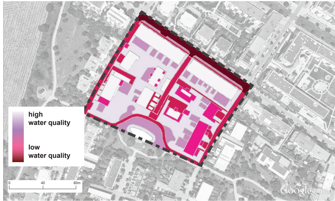
Figure 27 (top right): This figure represents the imperviousness and water quality seen at Site C in Riselfeld, Freiburg. The primary use of green roofs on buildings in this study site greatly reduce the amount of impermeable hardscape on the site (Created by author, Original map data: Google Earth, 2016c).
