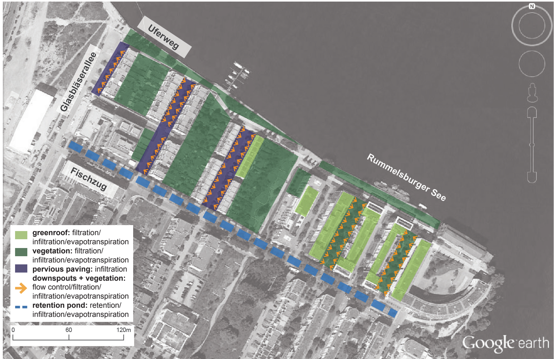
Figure 11: This diagram summarizes the general water management schemes on Site A as also represented with photographs and descriptions (Created by author, Original map data: Google Earth, 2016b).
