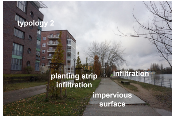
Image 15: The ground floor of typology 2 is raised higher than the Uferweg pathway creating a bowl like effect with the central open space to make sure all water associated with the building plot is treated on site. The public amenity space along Uferweg includes some vegetation and impervious paving, thus could be redesigned to incorporate more effective surface water management approaches.
