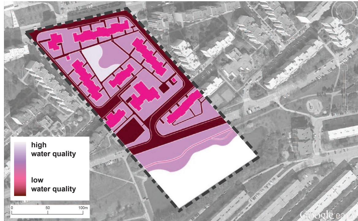
Figure 33: This diagram represents the land cover at Černý Most based on a typical typological block. The diagram shows land cover in terms of the water quality upon interaction with said land cover. This study allows for the estimated calculation of peak discharge runoff on the site. A similar study was done with the precedent Sites A, B and C. (Created by author, Original map data: Google Earth, 2016d).
