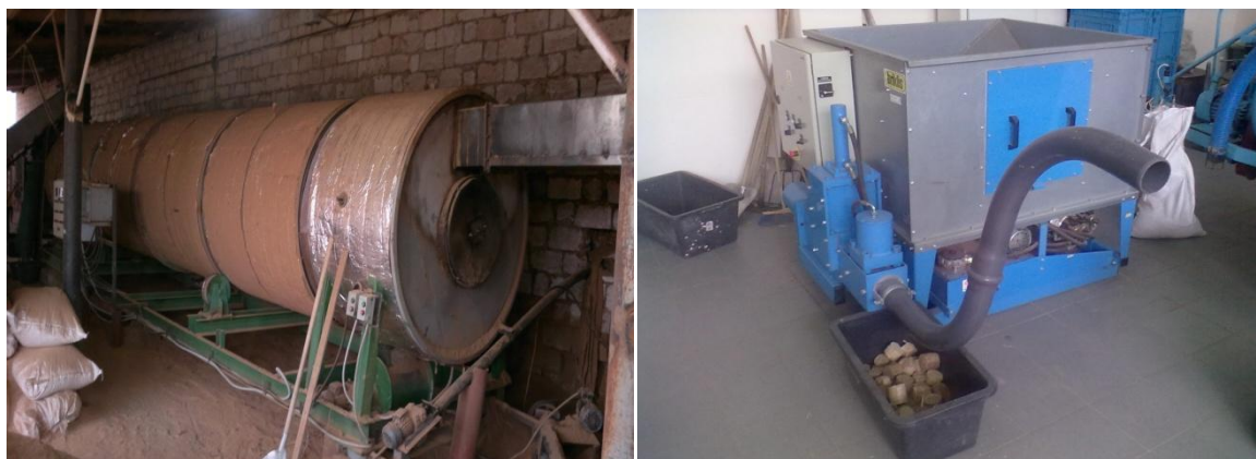
Figure 6.: (left) Drum dryer; (right) Briquetting press Brikliis BrikStar 50/12
