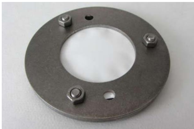
Obr. 8: POCIS – Polar Organic Chemical Integrative Sampler (Grabic a kol., 2015)
