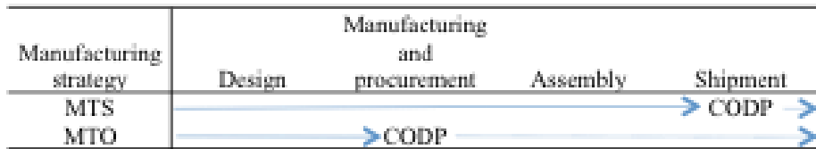
Figure 2.4 CODP in MTO and MTS manufacturing strategies (based on Sjobakk, Thomassen, & Alfnes, 2014)
