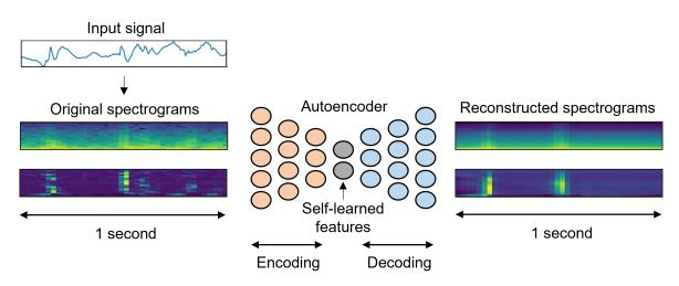
Figure 8: A schematic example of an autoencoder. Input data passes through the encoding layers, and the autoencoder extracts the self-learned features. In the reconstruction process, the features are propagated through decoding layers to produce an output.
