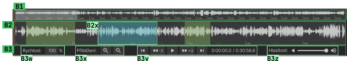
Figure 4.5: Decomposition of the player. The minimap is in B1. The waveform in B2 and it contains a region in B2x. Controls in B3 comprise the speed control in B3w, the zoom control in B3x, the playback controls in B3y, and the volume control in B3z.
