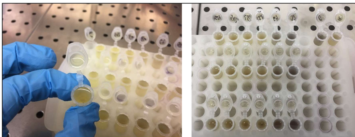
Figure 10. Broth macrodilution volatilization method MIC determination: the results are evaluated visually after coloring of living bacterial colonies with MTT dye
