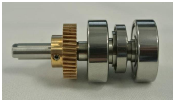
Figure 8: Eccentric cam shaft with worm gear
