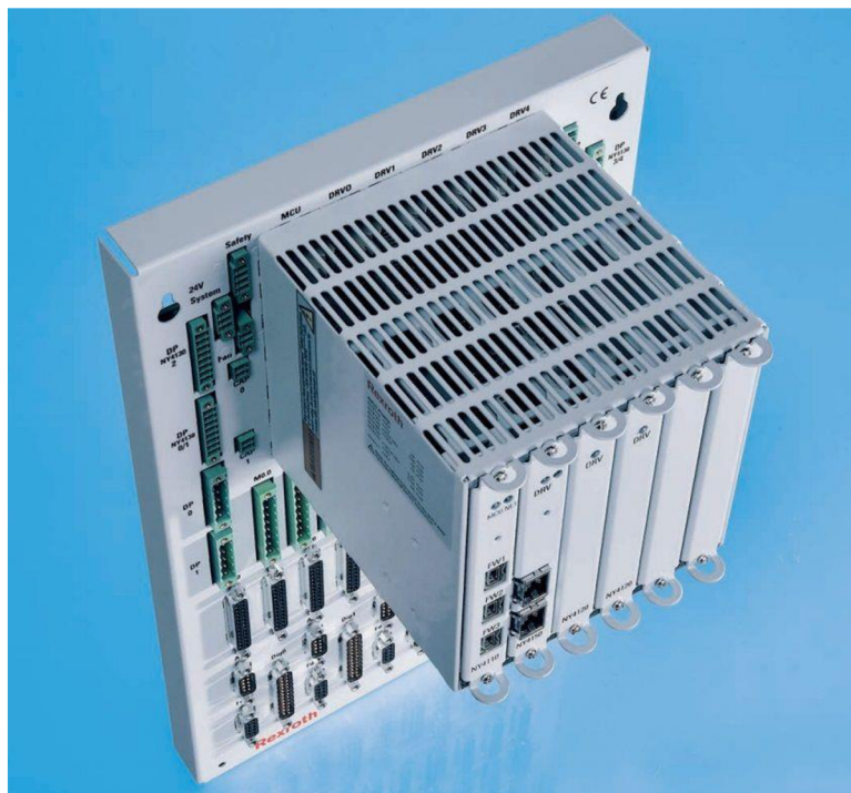
Figure 15: NYCe 4000 motion control unit. [13]
