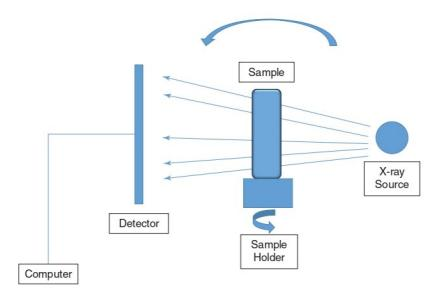
Fig. 2.1: Components of the micro-CT. [34]
