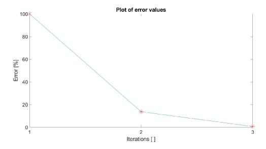
Fig. 6.13: Error between estimated shape and other shapes was computed after each iteration in GPA. The algorithm stops, once the error is below a threshold. In most cases, two iterations should suffice, according to Bookstein [5]
