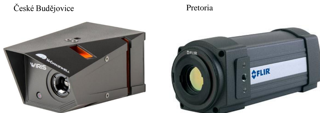
Figure 6: The thermographic cameras used in the experiment. From: WORKSWELLWIRIS, https://workswell.cz ; and FLIR SC325 Thermal Camera, https://www.instrumart.com
