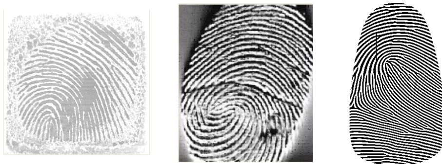
Figure 6.2: Real fingerprint images – oiled finger, hair on the sensor and simulated synthetic image.
