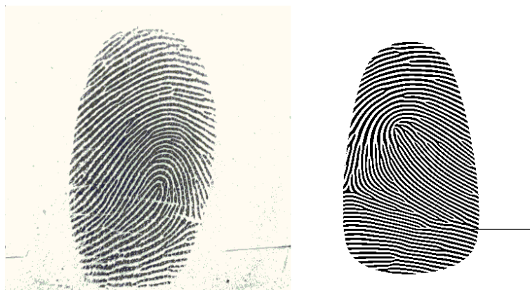
Figure 6.1: Real (left) and simulated (right) fingerprint from damaged sensor.
