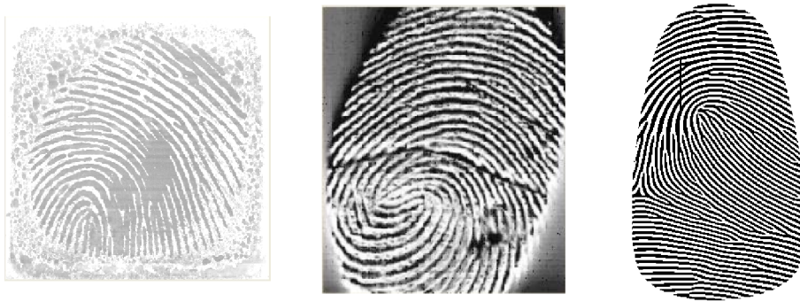
Figure 6.2: Real fingerprint images – oiled finger, hair on the sensor and simulated synthetic image.
