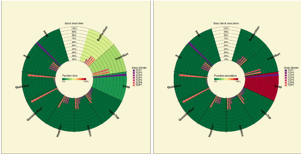
Figure 6.3: A visual interpretation of the collected basic block data, showing that the exclusive time spent in BadPartition function is significantly higher than any other function, indicating the source of the performance issue. The large version of these images can be found in Appendix B.
