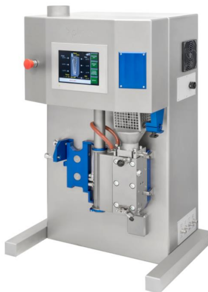
Obr. 3.3 Mikro compoundér Xplore MC 15 HT [32]
