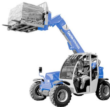
Figure 4.1: Telehandler GTH TM -5519 produced by GENIU [ www.robinrents.com/ ]
