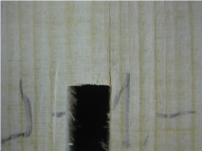
Figure 32: Detail of failure after loading test
