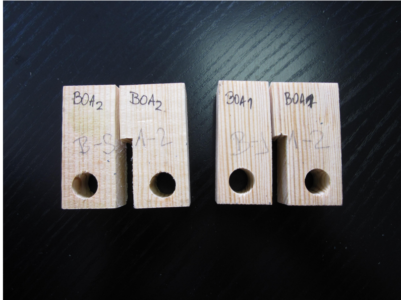
Figure 34: CT specimens after the test
