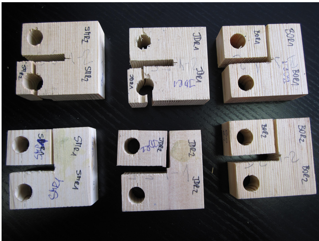
Figure 37: Broken CT specimens loaded in radial direction
