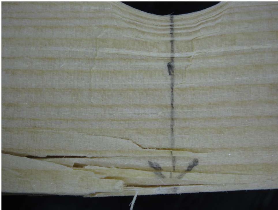
Figure 20: Local damage of Speciman 2 after bending tests
