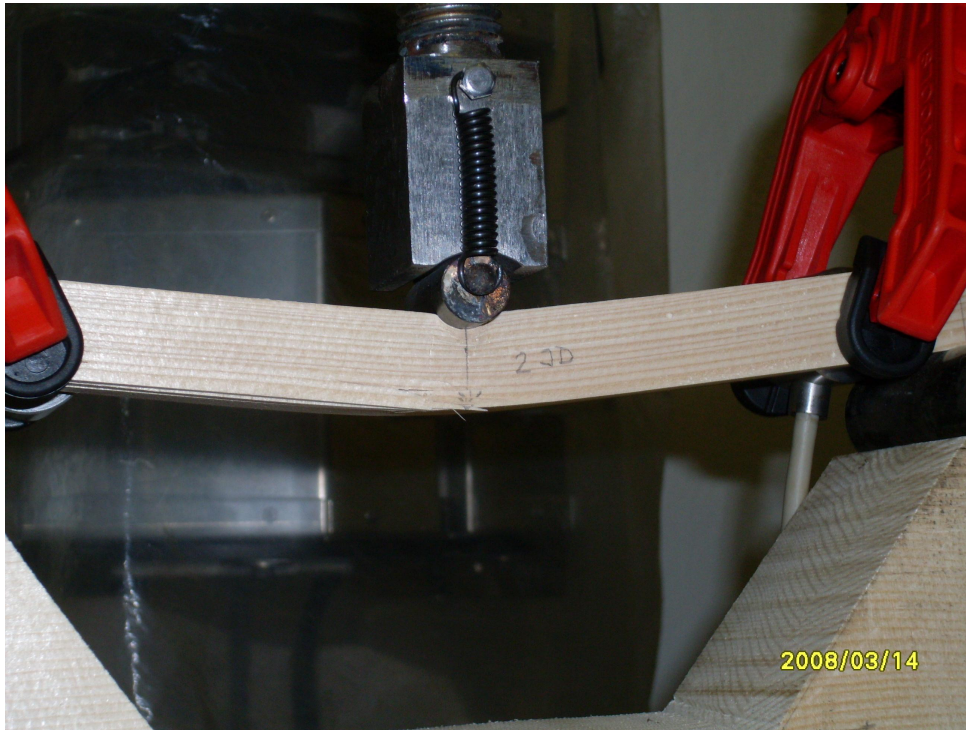
Figure19: Speciman 2 after bending test
