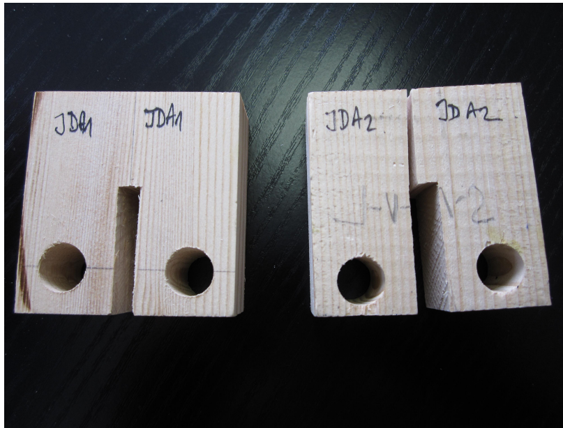
Figure 28: CT specimens after the test
