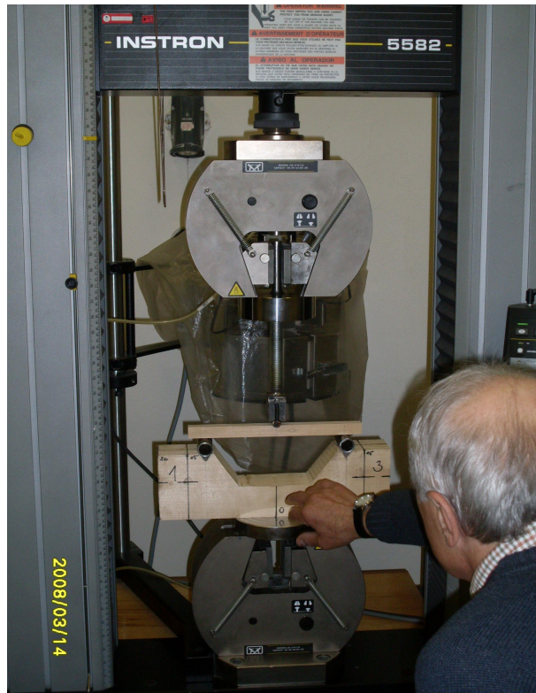
Figure 14: Preparation of specimen on INSTRON testing machine
