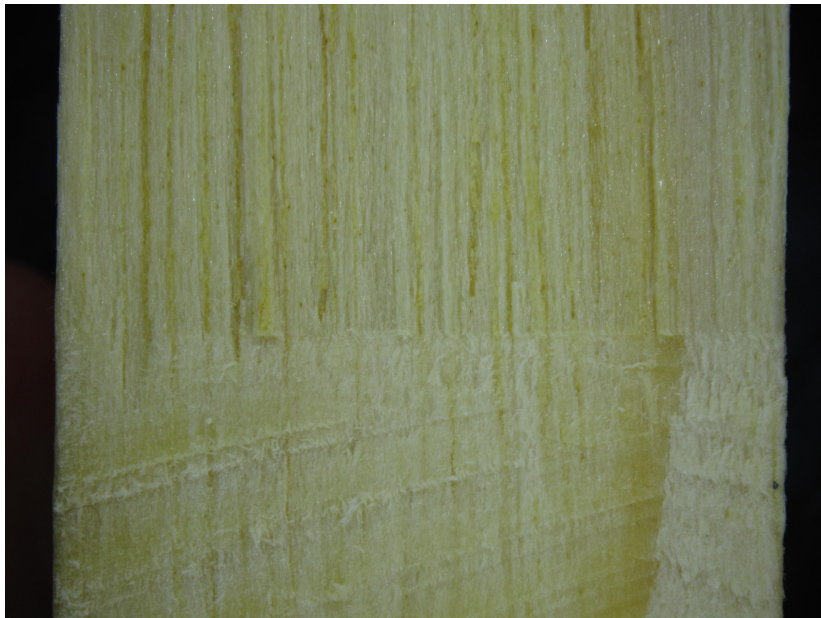
Figure 35: Detail of fracture area, specimen Pine A2
