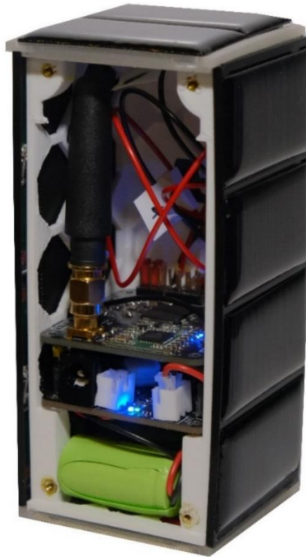
Figure 28: Detail on the PocketQube Electronics and inner structure
