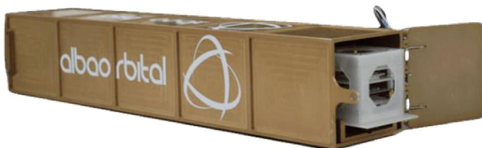
Figure 3: AlbaPod PocketQube deployer [29]
