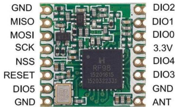
Figure 18: RFM98 communication module with pinout
