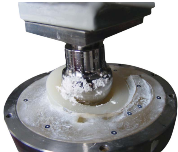
Figure 8. Validation test by hip pendulum.
