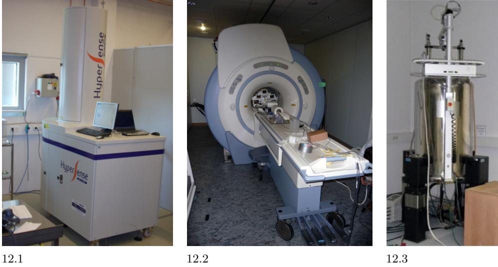
Figure 12: The hardware equipment at GE Global Research centre in Garching bei München used for the experiment. 1) Oxford Instruments HyperSense™ DNP polarizer. 2) The GE Signa® EXCITE™ 3.0 T MRI scanner. 3) Bruker AVANCE III 600 "Laurel" located at Bavarian NMR Center (BNMRZ)
