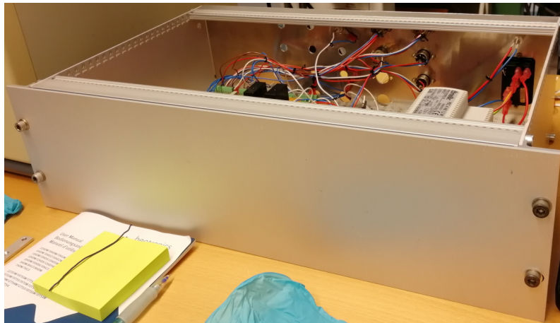
Figure 4.16: Front view of control unit housed in a 19-inch rack.
