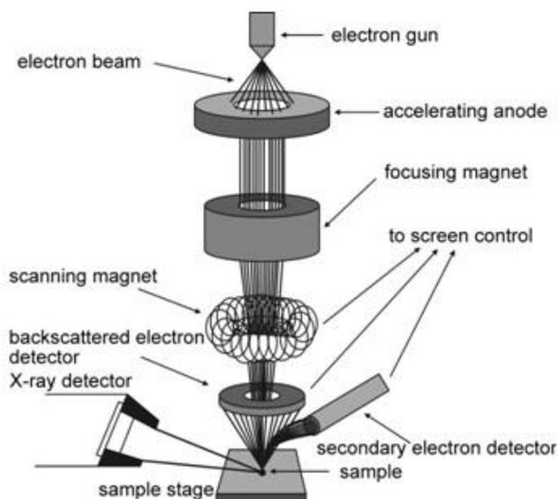
Figure 5: Setup of a scanning electron microscope, adapted from [33]
