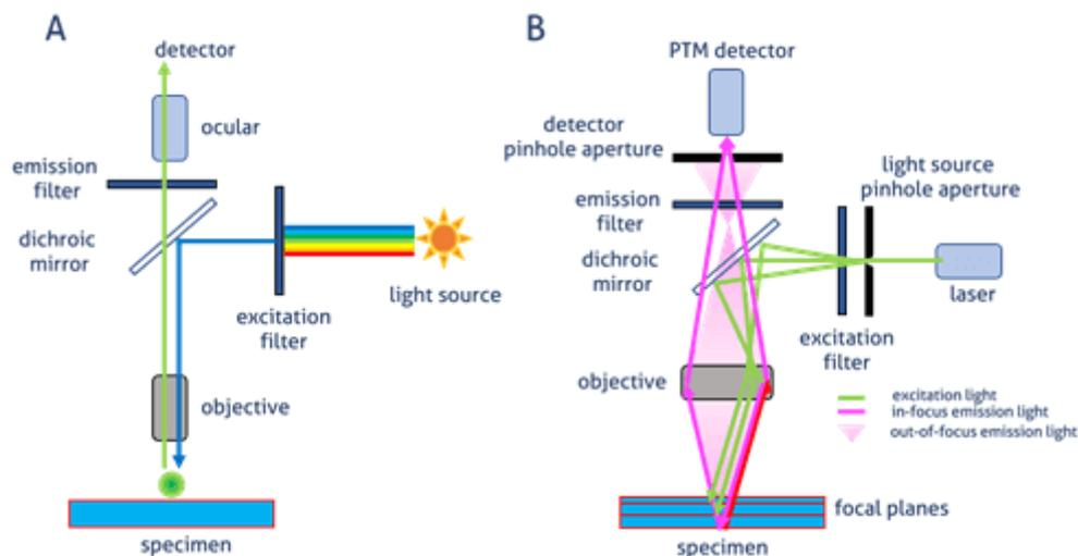
Figure 6: Schematic setups of a widefield fluorescence microscope (left) and a confocal microscope (right), adapted from [39]
