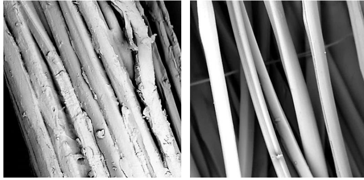
Figure 2.2 SEM images of silk fibres before (left) and after (right) degumming (SEM magnification 2 kx)
