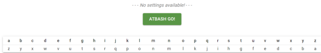
Fig. 4.4: Detailed view of the Atbash cipher settings.
