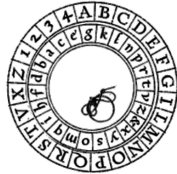
Fig. 1.5: Alberti cipher disk [6].
