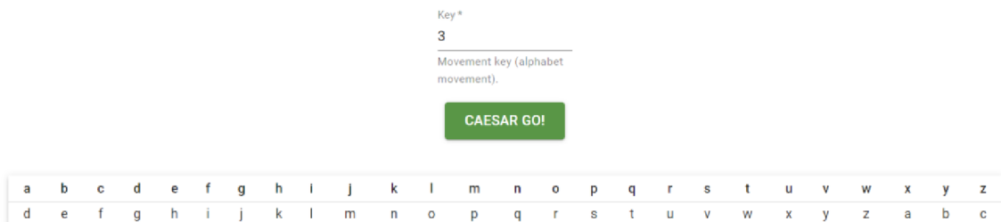
Fig. 4.5: Detailed view of the Caesar cipher settings.
