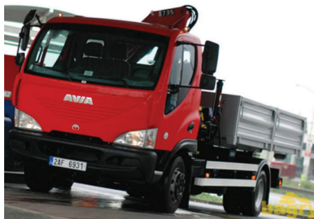
Obr. 56: AVIA D120 - 185 L s hydraulickou rukou HMF 735-K2 [7]
