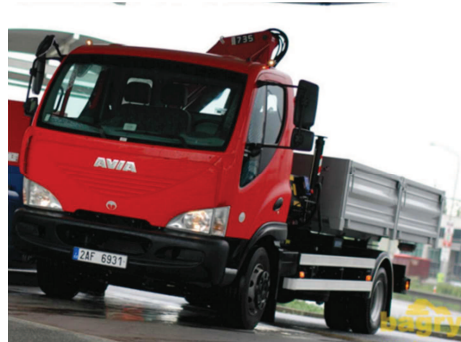
Obr. 26: AVIA D120 - 185 L s hydraulickou rukou HMF 735-K2 [7]
