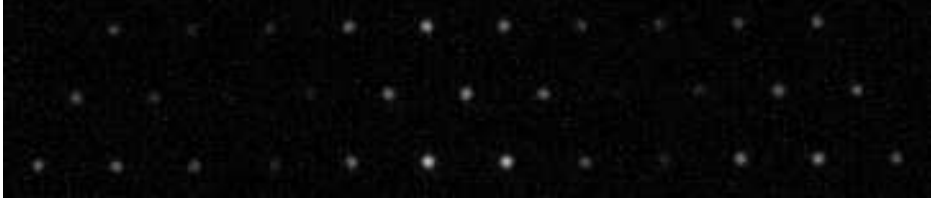
Figure 4.8: CCD image for the state \rho_{\text{coh}}^{\text{true}} . The relevant part of the SH readout used for the beam reconstruction is shown. Contributions from the individual SH apertures are indicated by bright spots, with each spot made up of multiple pixels. Note that the two void regions correspond to the phase singularities of the state \rho_{\text{coh}}^{\text{sup}} . This hints that \rho_{\text{coh}}^{\text{true}} \approx \rho_{\text{coh}}^{\text{sup}} .
