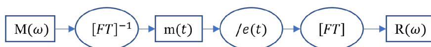
Figure 5.6: Schematic depiction of the deconvolution algorithm used to obtain undistorted slow scan spectra.
