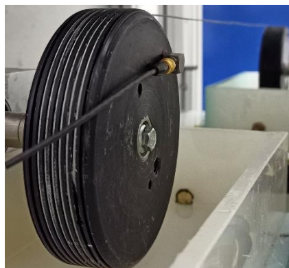
Figure 3-3 accelerometer positioned on pulley
