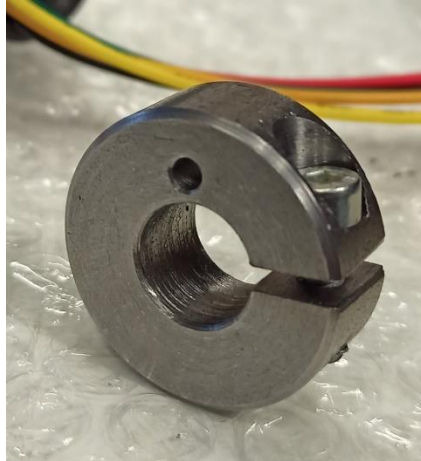
Figure 5-5 ring used to connect the shaft and the wire with hanging mass
