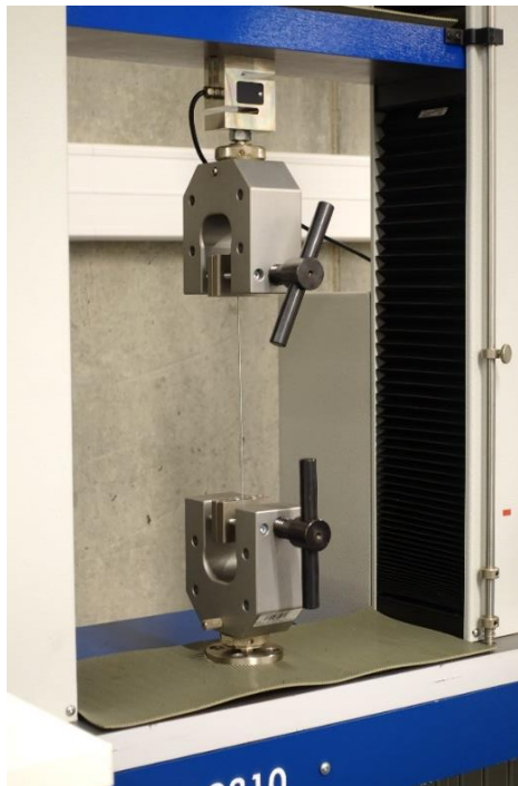
Figure 3-1 cable of length 200mm placed in a Universal testing machine
