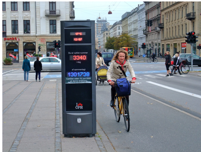
Figure 4.1: Automatic bicycle counter in Copenhagen, Denmark. Source: [11]
