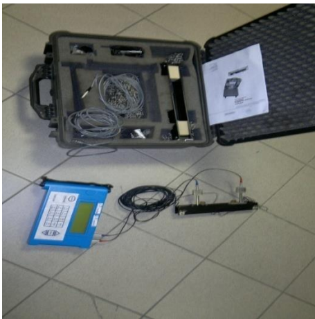
Picture 2.19. – Portable ultrasonic flow meter UFM 610P Krohne
