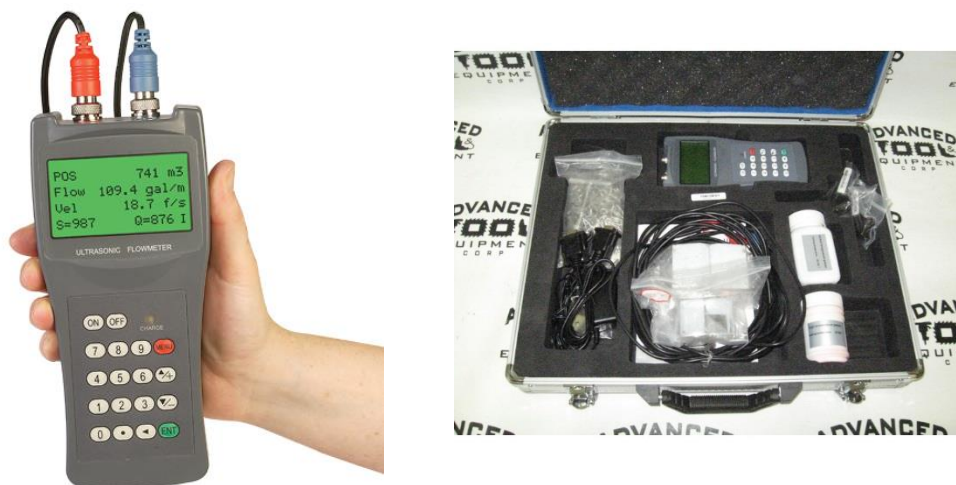
Picture 2.20. – Left ultrasonic flow meter FDT-21, right flow meter case
