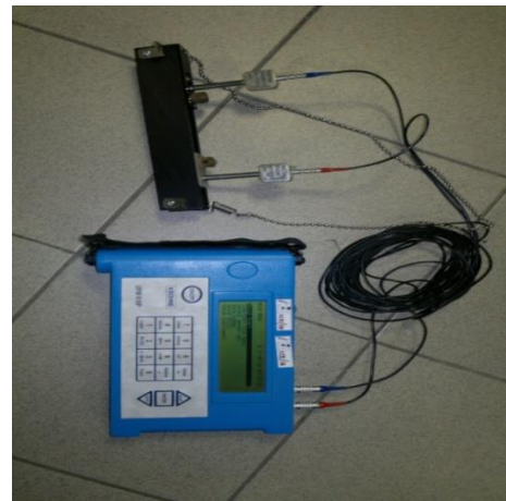
Picture 2.19. – Portable ultrasonic flow meter UFM 610P Krohne
