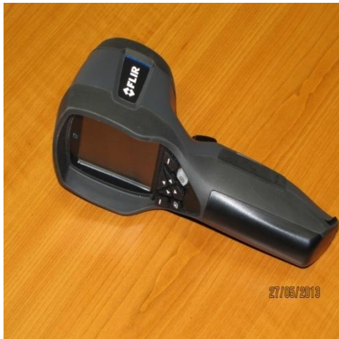
Picture 2.16. – Thermography camera Flir i7.
