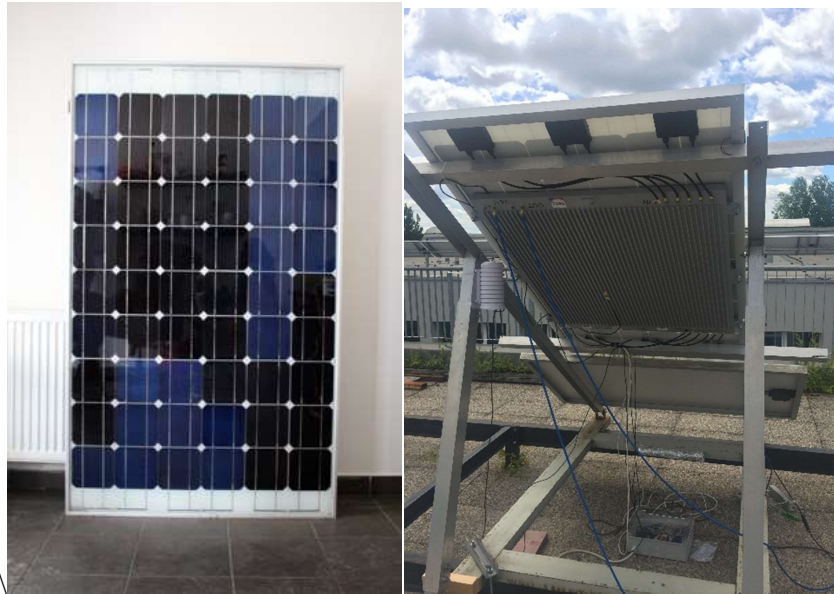
Figure 12. Front and rear side of the PV-battery module prototype
