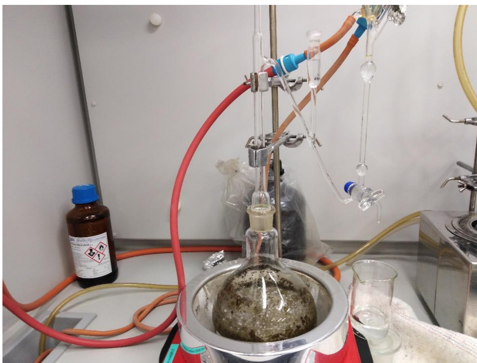
Picture 10: Hydro-distillation extraction of essential oil from the sample n.1
