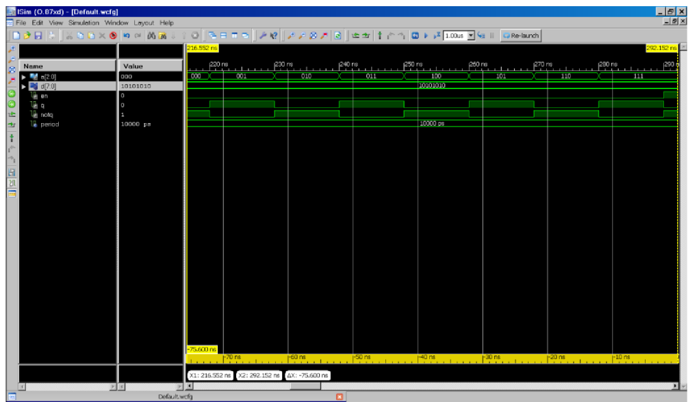
Obr. 6.4: Simulace obvodu 74151, multiplexoru.
