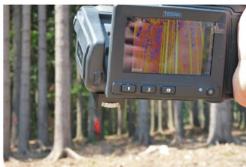
Fig. 9. A thermal camera showing temperature measurement from the newly created forest edge.
