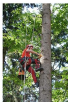
Fig. 10. A tree climber measuring tree stem temperature by using infra-red thermometer.
