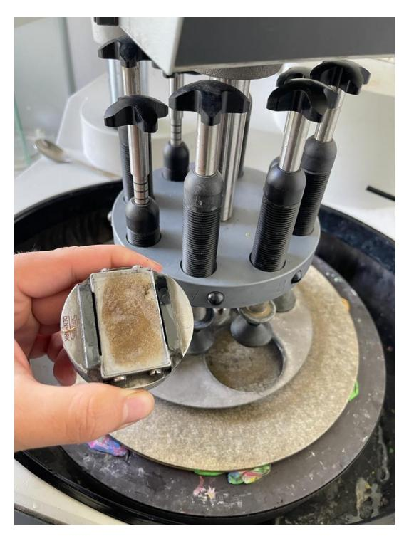
Figure 6 thin section polishing machine
