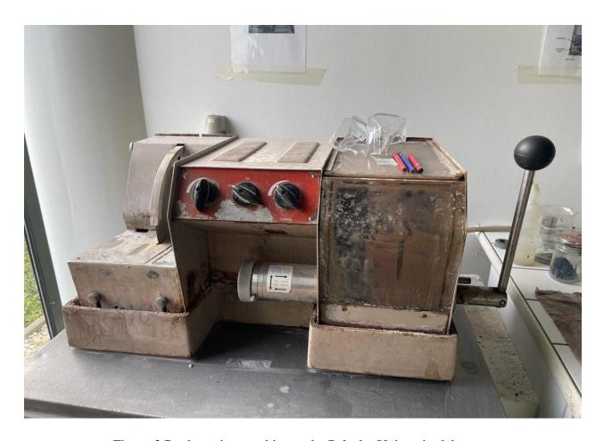
Figure 3 Rock cutting machine at the Palacky University lab
