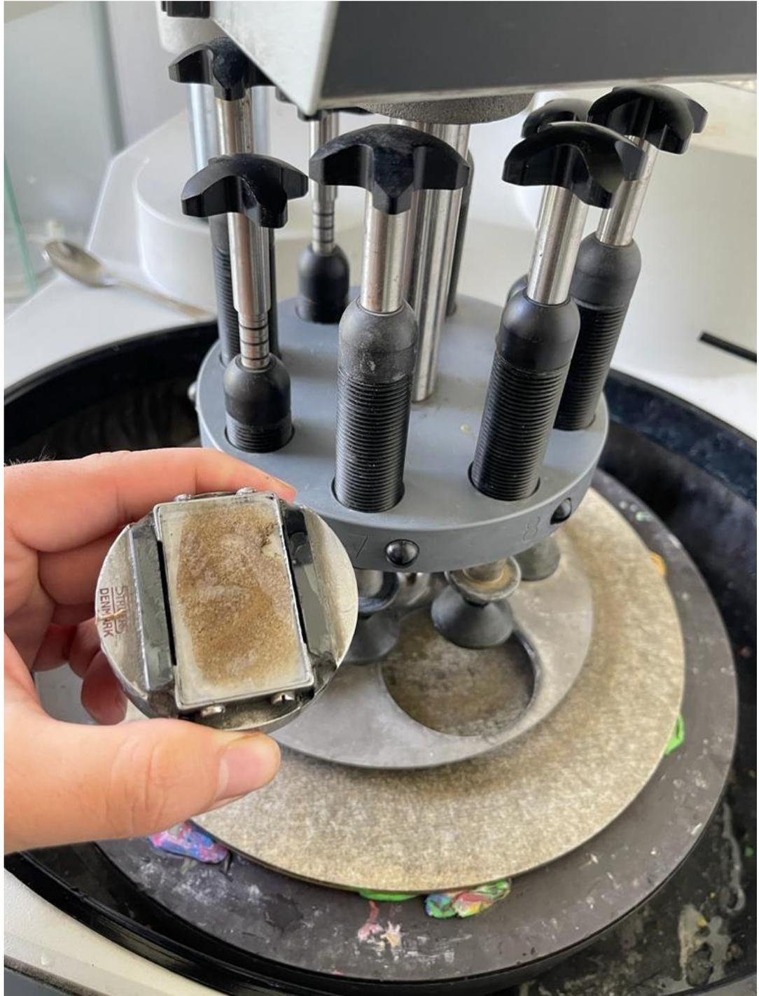
Figure 6 thin section polishing machine
