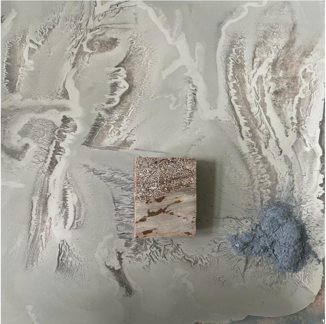
Figure 4 rock sample with polished and grinded with glass plate and powder
