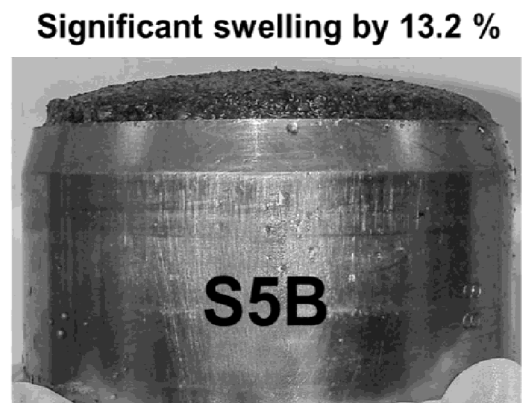
Fig. 2.2 The swelling effect in case of soil samples (CS – control non-clayed soil; S2B – 2% biochar dose to non-clayed soil; S5B – 5% biochar dose to non-clayed soil); graph shows measured WHC values at saturation for non-clayed soil; different letters following means (n = 5) indicate significant differences between treatments (Tukey HSD test at \alpha = 0.05 ).
