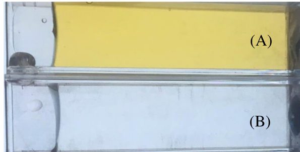
Figure 2-9 Methyl orange dye before (A) and after (B) photocatalytic degradation
