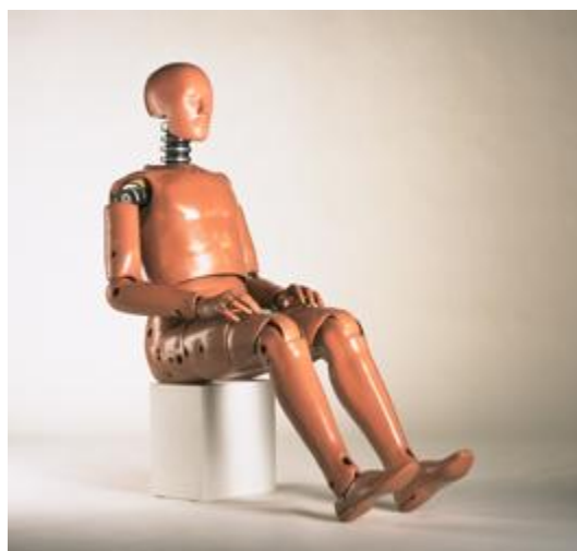
Obr. 15 Hybrid III 50. percentile Muž [16]
