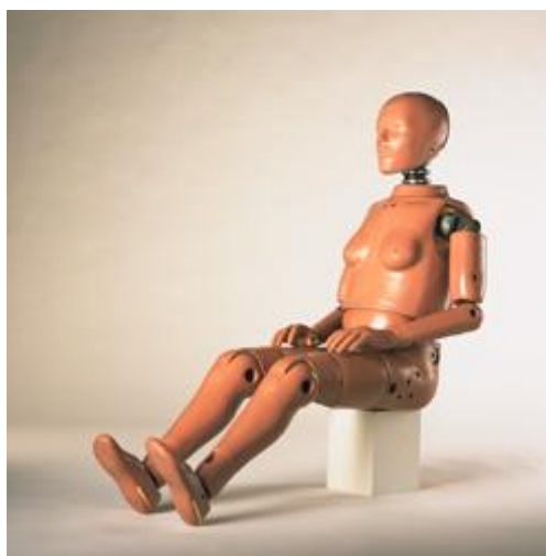
Obr. 14 Hybrid III 5. percentile Žena [16]
