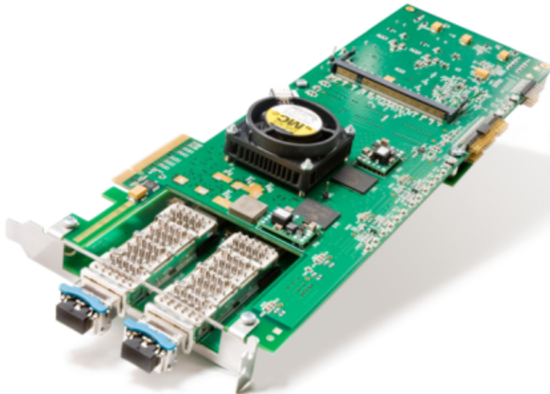
Figure 3.6: COMBOv2 Mother Card with Attached 2x10 Gbit/s Interface Card [31]
