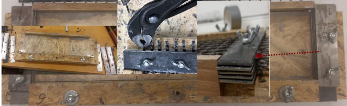
Figure 3.6 Photograph showing the detail components of the mold system of dimension 400 \times 100 \times 15 \text{ mm}^3 .
