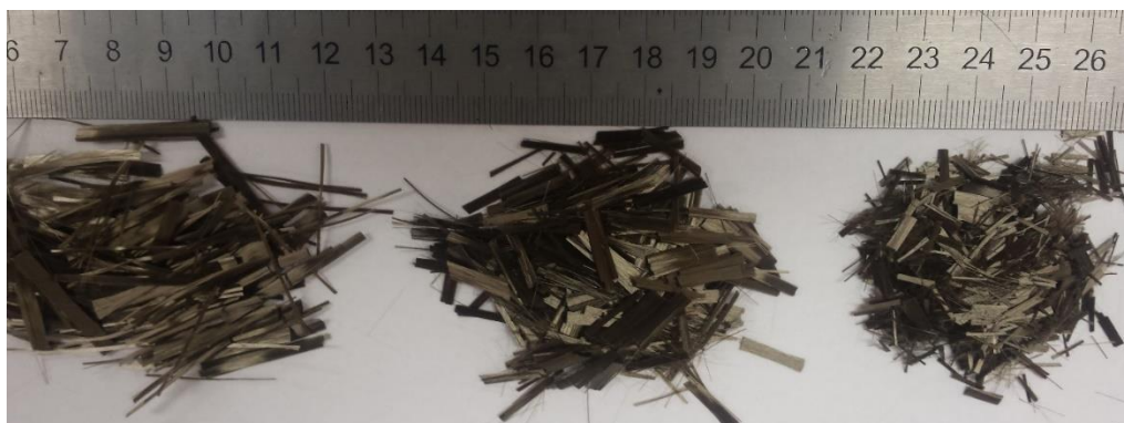
Figure 3.2 Three types of the chopped basalt fibers (BF) with different fiber lengths used in this work, from left to right: fiber length of 24 mm (24 mm BF), the fiber length of 12 mm (12 mm BF), the fiber length of 6 mm (6 mm BF).
