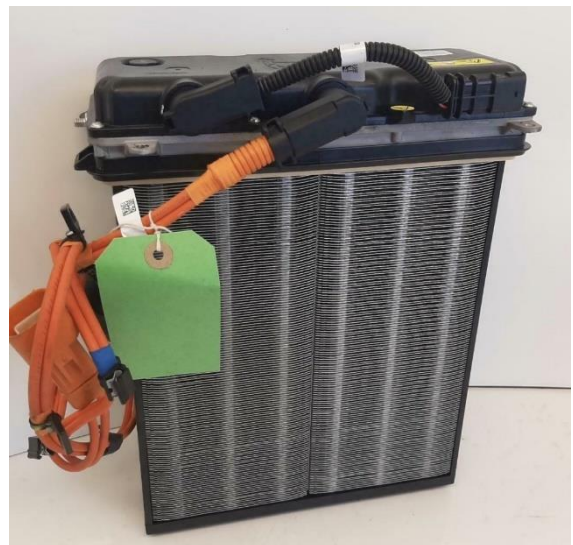
Figure 15. PTC air heater used by Tesla Model 3 [73]
