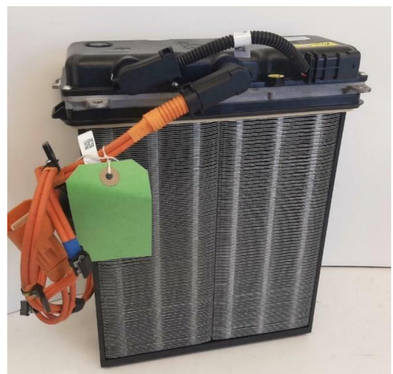
Figure 15. PTC air heater used by Tesla Model 3 [73]
